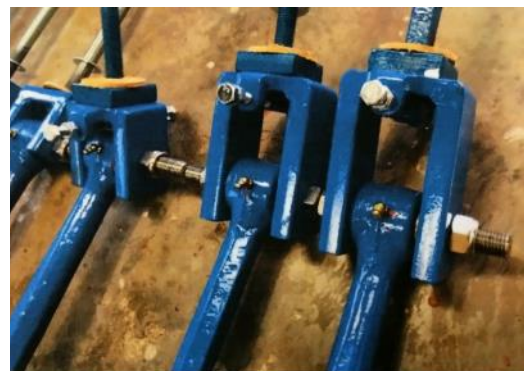
Refurbished adjustable staples—similar to the work being done on St Matthew's bells. The staples hold the clappers in place.
